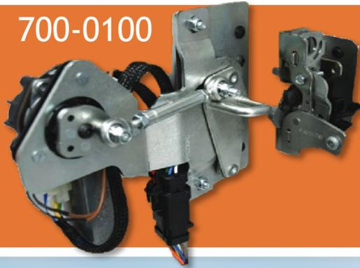
TriMark's Power Cinching Strike is designed for large and heavy doors that have difficulty closing due to higher door seals, air compression or pre-bowed glass. The cinching function is completed in a slow and smooth operation using a robust electric motor drive instead of a door slam
