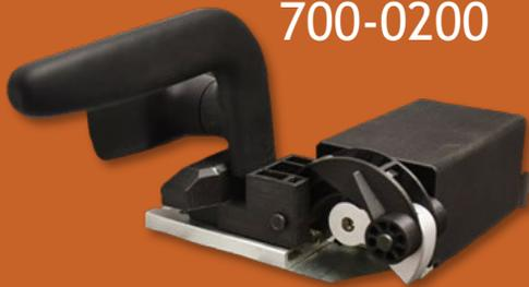
The Power Vent Window System is designed for large vent windows that utilize a quarter turn window handle. Coupled with a state sensing door latch, the window vents when the entrance door is opened, providing ease of door closing by reducing air compression
